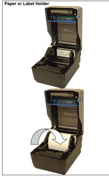
Allows loading of paper, including adjusting of width of paper holder to match paper size.
